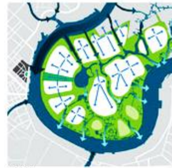
Hydrology Thu Thiem acts as a natural filtration system using water-receiving landscapes and enhanced plant species forming an open system that allows infiltration and fluctuation of tides from the Saigon River
