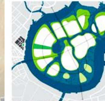
Storm Water Management Extreme high tides and flooding are handled through raising development areas to a minimum of +2.5m elevation and allowing surrounding landscapes to "receive" water (flood)
